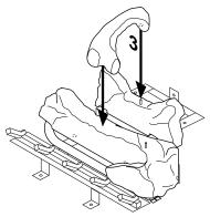
Figure 52 - Installing Log No. 3
